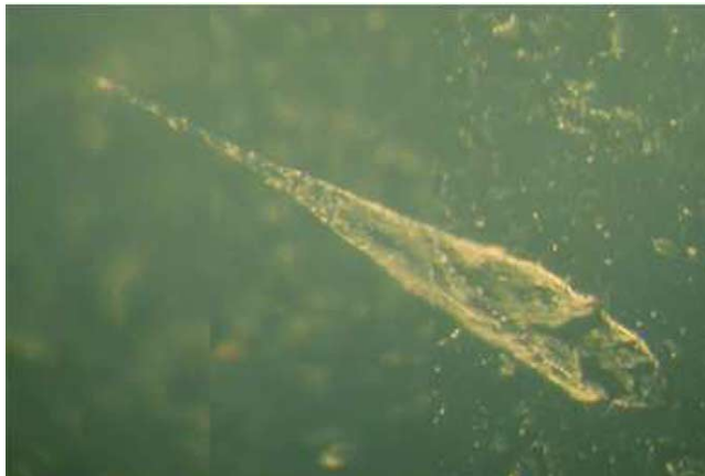
Fig. 1. Carrot shaped track found in aerogel exposed on the Mir Space Station. The projectile entered the aerogel from the lower right and is found at the upper left hand corner of the image.
